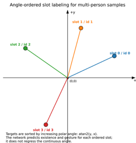
Fig. 9: Angle-ordered slot labeling. Slot IDs are assigned by sorting persons according to \text{atan2}(y, x) around
