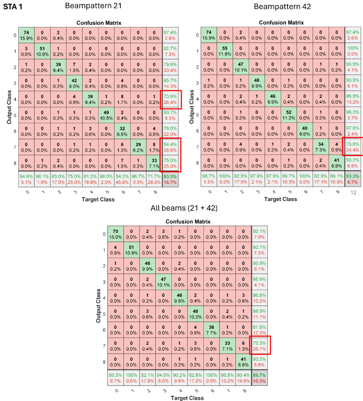
Figure 11: Selected confusion matrices for the motion detection (with up to X=8 subjects): (a) STA i=1, beampattern code k=21; (b) STA i=1, beampattern k=42; (c) STA i=1, beampatterns codes k=21 and k=42; (d) STA i=4, beampattern code k=21; (e) STA i=4, beampattern k=42; (f) STA i=4, beampatterns codes k=21 and k=42.
