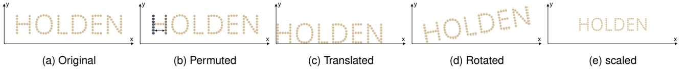
Figure 4: Different features of point clouds which affect the way they need to be processed are shown in this figure. To simplify visualization, the text "HOLDEN" is shown in the form of a point cloud in a 2D space.
